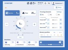
Specimen head position memory function allows specimen head to be reset to memorized position with just one touch.
